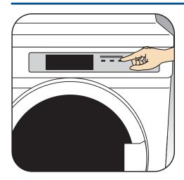
**5.** The dryer will stop if the door is opened during the drying cycle. To restart the dryer, close the door, reselect the cycle and press start.
